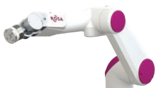
Figure 1. Illustration of the ROSA ONE Brain and Spine robotic arm.
