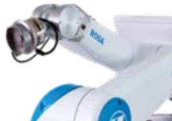
Figure 2. Illustration of the ROSA Knee robotic arm.
