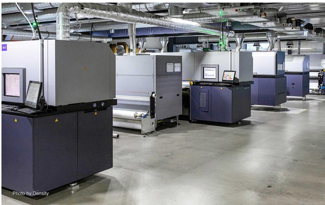
The print room of the Moss site in Lennestadt (Germany), with Durst 1.6, 3.2 and 5-metre printers that feature either UV-curable or sublimation inks.
