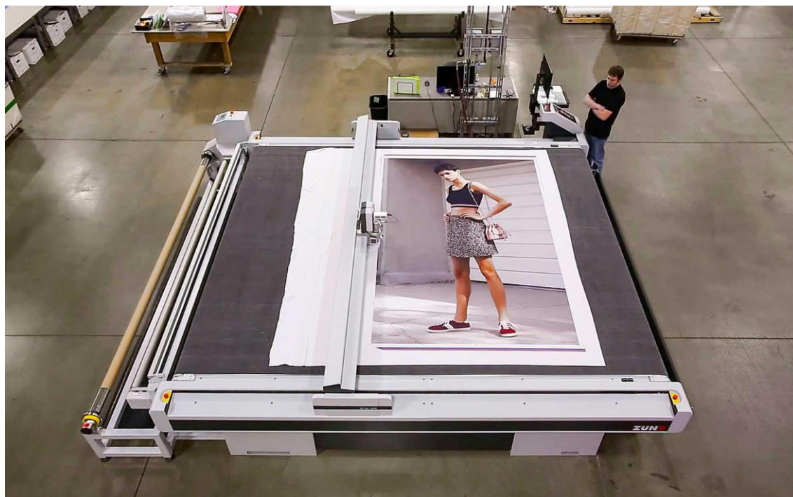
To cut fabric, Moss mainly uses 3.2-metre-wide Zünd cutting tables, configured with a conveyor belt, unwinder, and rotary knife tool.
