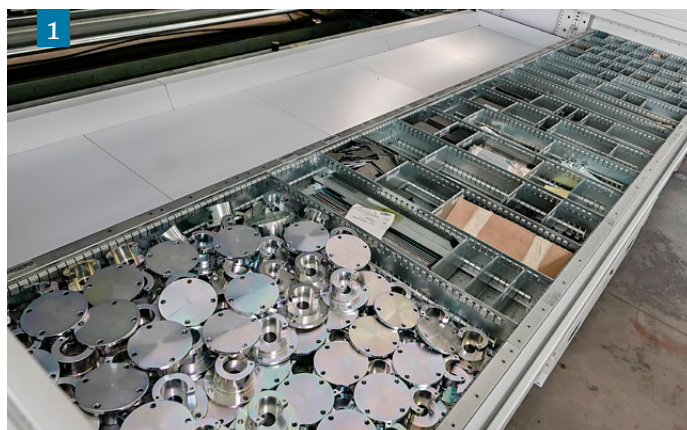
1) The four vertical lift modules installed in the company contain and make available to technicians all the small components necessary for assembly. 2) Rollers stored in the semi-finished products warehouse, before being moved to the final assembly area. 3) The area dedicated to the final assembly of large format machinery.
