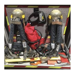
One design aspect example of the clean cab concept is removing the SCBA from the cab and instead placing it in exterior compartments. To further reduce exposure, this gear is typically put into plastic bags following decon until it can be safely dealt with - The Decon<sup>TM</sup> Bag aims to take this one step further in regards to protection and also offering a reusable alternative to trash bags.
